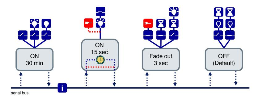
→ "Ignition on" data should be sent from state "ON 30 min" to state "Fade out 3 sec" through state "ON 15 sec" which is bypassing the timer
